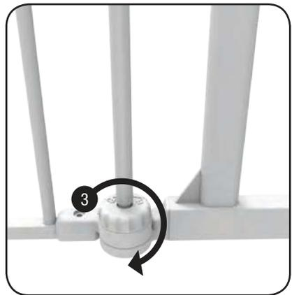
Turn the base knob in a clockwise direction to lock panels.
