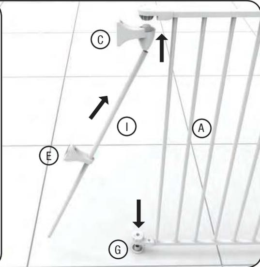
NOTE: Place Lower Wall Bracket (E) over Corner Tube (I) before assembly.
