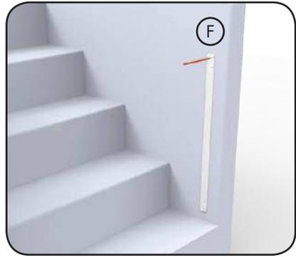
1. **Screws provided are for mounting directly into wood. If mounting into brick, drywall or other surfaces use appropriate hardware, note that drilling a pilot hole may be necessary.** Hold guide 1 (E) vertically and completely outstretched against mounting surface with the end marked "FLOOR" even with the floor. **Note: leave 2cm between guide (F) and the edge of the opening to ensure gate won't overhang edge.** Mark screw hole positions. Remove the template. Repeat process for Guide 2 (F).
