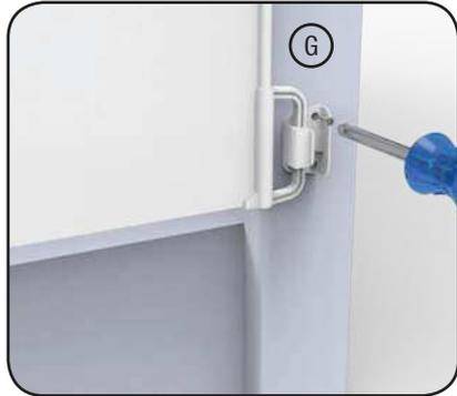
2. Align each mount in its correct position, use a Phillips screwdriver to tighten screws till each mount is secure.
