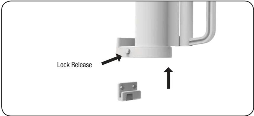
To remove gate from the mounts push and hold the lock release button while sliding the gate upwards.
