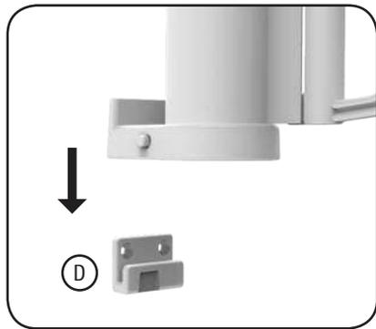
3. Attach Gate Assembly to the Gate Mounts by aligning the gate directly above the mounts and sliding straight down over mounts. Check that the Gate assembly is flush against the wall and is locked firmly in place.
