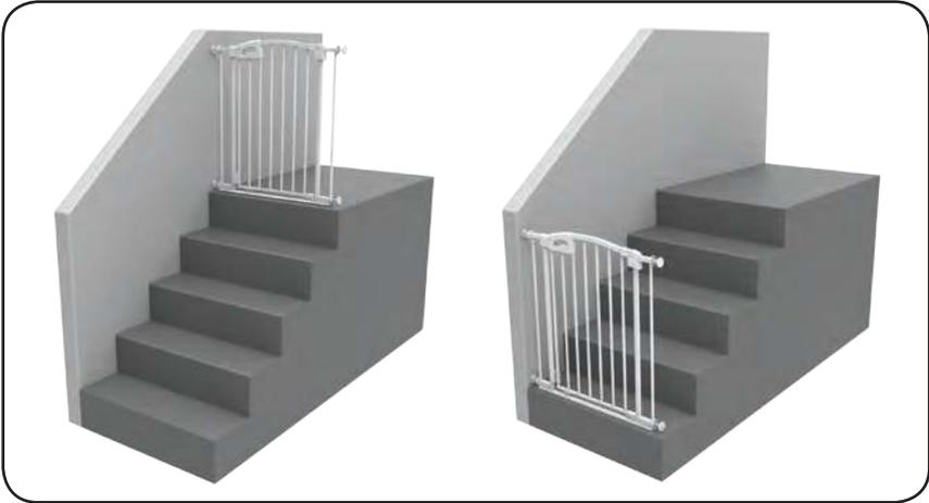
If using gate on a stairway, it must be placed either on the top step or on the lowest step at the bottom.
