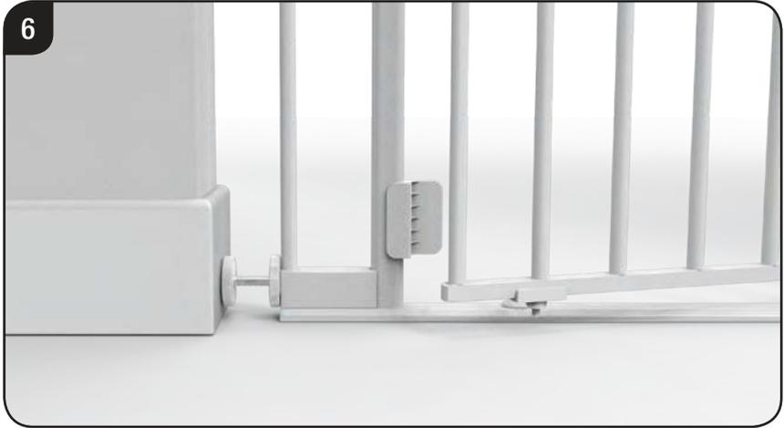
6. Determine which direction the gate should open. **For the top of stairways, gate should never open out over stairs.** Screw in Swing Direction Control piece opposite to the desired opening direction. Use images below as a guide.
