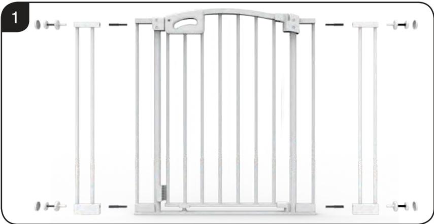
1. Measure the space to be enclosed, you may need to use extensions. Extensions are available through [www.permachildsafety.com](http://www.permachildsafety.com).
